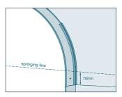
5 Nail or screw the long leg of the bead through the plasterboard and into the particle board every 230mm (maximum centres) and no closer than 70mm below the springing line.
