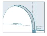
Nail or screw the end of the reveal strip to the wall studs at least 50mm below the springing line on each side of the arch.
